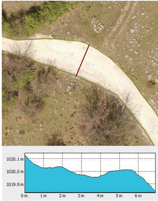
Picture 8. The maximum width of the road and its cross-section profile
